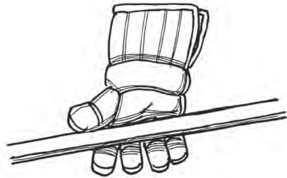
Figure 3-2. Determining the size of the shaft.
